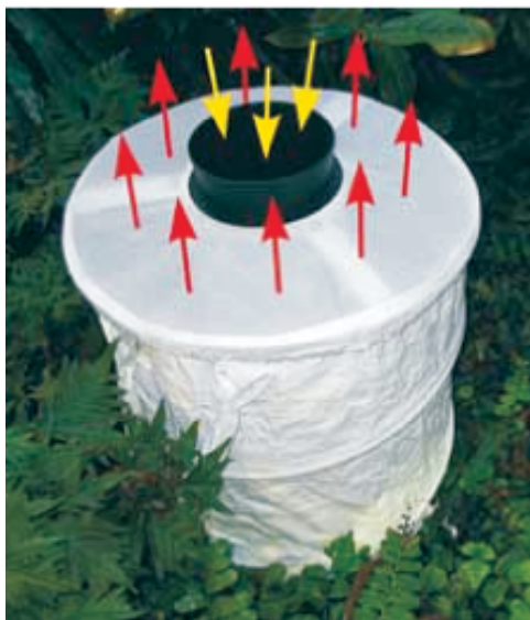
Fig. 1: the BG Sentinel-Trap. Mosquitoes flying in trap vicinity are attracted by a dispenser which releases a combination of components found in human skin and are captured in the black centered catch bag (yellow arrows). The air exits the trap through the large surface of white gauze (red arrows), generating ascending currents
