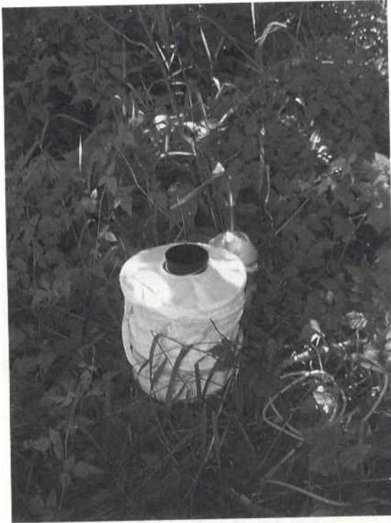
Fig. 1. The BGS trap with dry ice container and tube.
