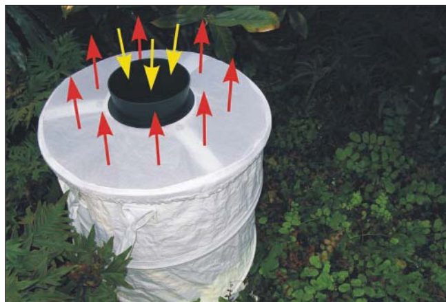
Fig. 2: Photograph of the BG Sentinel®. The yellow arrows show the direction of the drawn-in air, the red arrows the air loaded with the attractants which are emitted through the permeable fabric.
